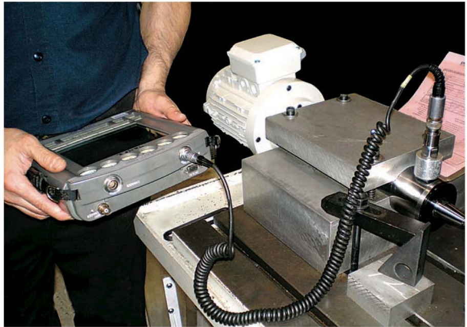
Comprehensive vibration analysis performed on a motorized grinding spindle.
