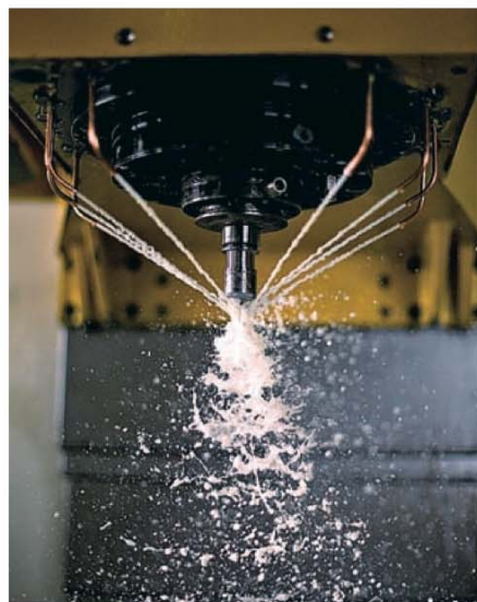
A high-speed spindle undergoing a coolant diagnostic test.
